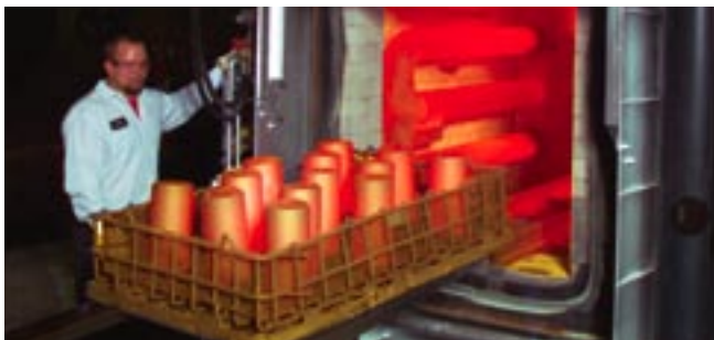
Atmosphere heat treating utilizing air, oil, water and salt quenching
